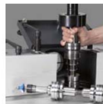
Moulder spindle quick change system
